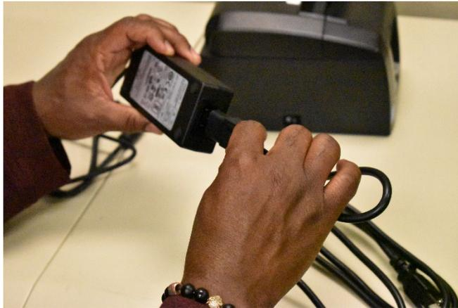
3. Plug the connector into the back of the printer making sure the arrow is on the top.
