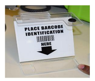
9. Attach the Photo ID Tray to the Poll Pad by sliding it on the mounting clip attached to the back of the Poll Pad.
