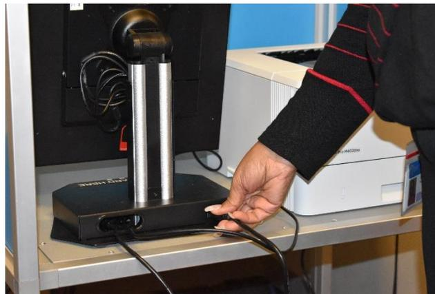
18. Carefully turn the BMD completely around so the screen faces you.
