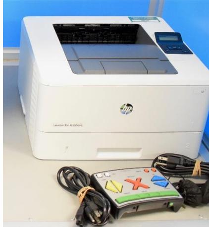
14. The BMD has three cords; two cords attached to the BMD – the ATI cord and the printer USB cord; and one power cord.
