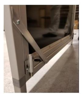
4. Lift the bottom panel of the booth up until it touches the bottoms of the left and right side.
