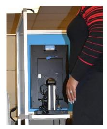
6. While holding the handle on the back of the BMD, slightly push the bottom of the BMD touchscreen forward to release the two cords secured behind the screen. Then sanitize the back of the BMD(Do not turn BMD around) and the cords.
