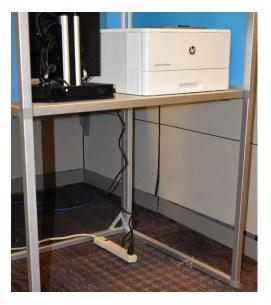
17. Take the BMD power cord previously removed from the black bag and plug into the BMD. Drop the opposite end of the power cord through the hole in the back of the voting booth and plug into surge protector.
