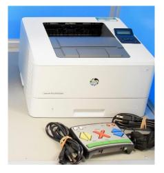
14. The BMD has three cords; two cords attached to the BMD – the ATI cord and the printer USB cord; and one power cord.
