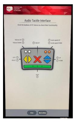
7. Once all green check marks are present on the screen, tap the 'Back to Menu' button at the bottom of the screen. Place the ATI unit and headphones behind the BMD.
