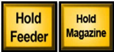
**Note:** The Hold Feeder and Hold Magazine buttons should now be lit up, indicating that they are not active. The Feeder “feeds” the VBM envelopes into the machine and is the red belt at the end of the “Magazine” belt that moves the VBM envelopes forward.
