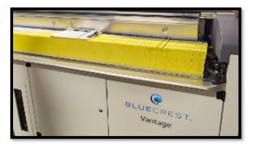
Note: Make sure the envelopes are loaded neatly and snug against the feeder belt.
