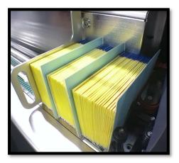
**Note:** If separator cards are not placed between the batches when running multiple batches at once, the batch will go to the Didn't Scan Tray Tag (pocket 19), forcing the team to run the envelopes through the machine a second time after the tray tag is printed.
