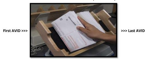
3. When loading envelopes on the Jogging machines, place envelopes **upside down**, with the colored bar at the top of the envelope facing the padding of the jogger.
