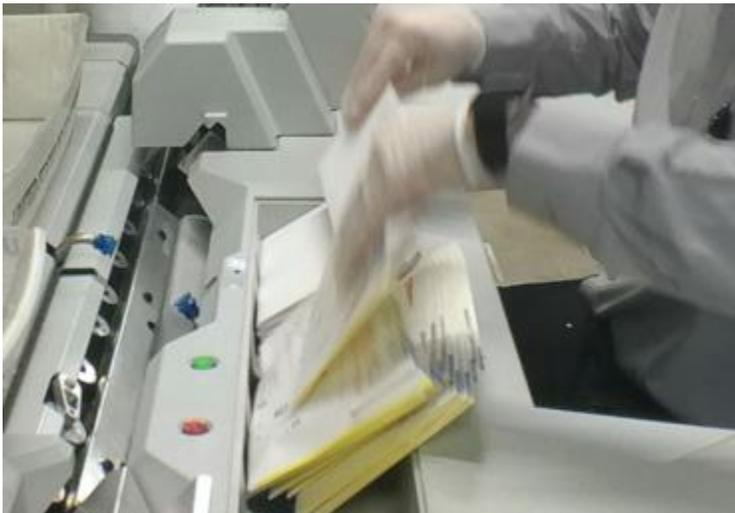
**Note:** Failure to pull the envelope directly up will cause the machine to believe that there is an error and stop the feeding process. If this happens, press the green button to continue.
