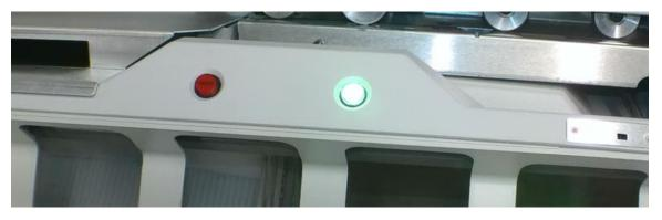
3. Press the green button to start the machine. It will begin to slice and feed envelopes down the path and open the envelope directly in front of you.
