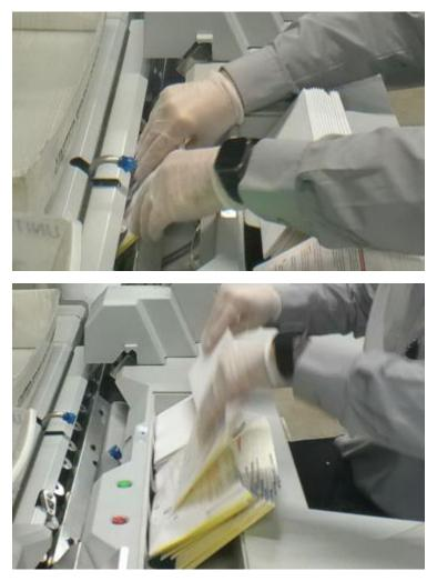
**Note:** Failure to pull the envelope directly up will cause the machine to believe that there is an error and stop the feeding process. If this happens, press the green button to continue.
