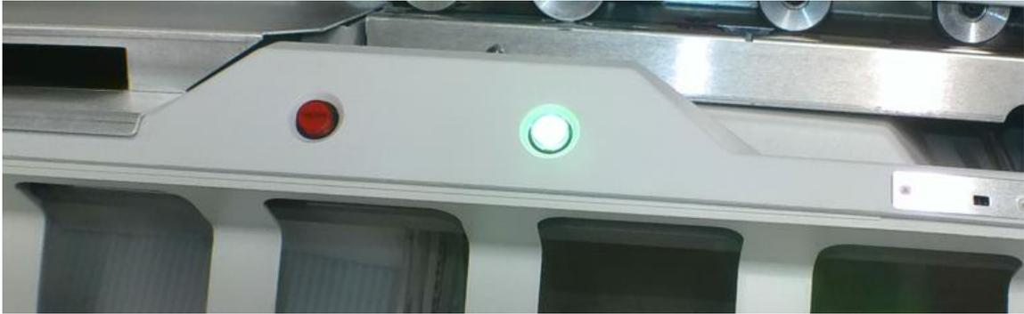
3. Press the green button to start the machine. It will begin to slice and feed envelopes down the path and open the envelope directly in front of you.
