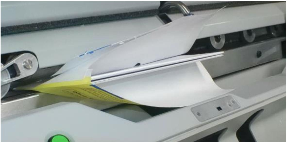
4. Use your left hand to grab and pull the envelope directly upward and your right hand to simultaneously remove the folded ballot cards, placing them in separate piles in the bin directly in front of you.
