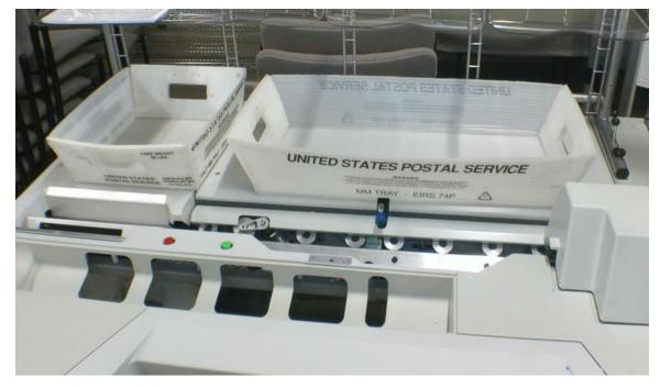
10. Move the tray tag insert from the Folded Ballot Tray to the Extracted Envelope Tray.
