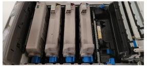
Open the printer and find the appropriate ink and replace the Toner and Drum
