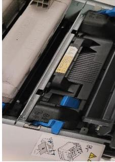
1. Open printer and replace fuser when it is cooled off.
