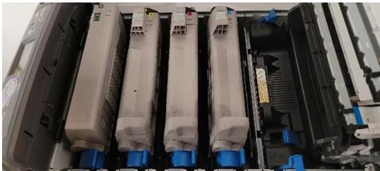
Open the printer and find the appropriate ink and replace the Toner and Drum
